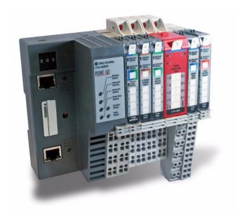
Each POINT I/O module mounts adjacent to the network adapter or another I/O module and removable terminal block (RTB) to connect all field-side wiring. The RTBs are part of the terminal base assembly. They are not included with the I/O modules and must be ordered separately.
