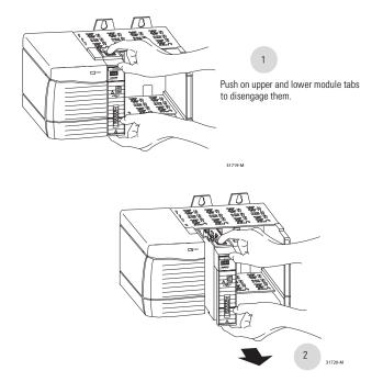
Slide module out of chassis.
