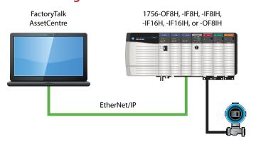
FDT Technology standardizes the communication interface between field devices and host systems to reduce integration efforts. FactoryTalk AssetCentre Process Device Configuration is enabled by FDT Technology.
