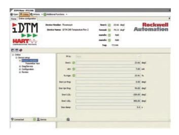
DTM device drivers can be obtained directly from the device manufacturer (for example, Endress+Hauser, Metso, Dresser Mason Neilson and others) for online configuration or for advanced device configuration. The iDTM can also be used when the device manufacturer does not supply DTMs for asset management solutions.
