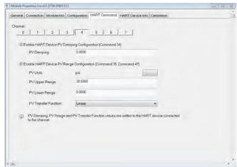
The Command Tab for the 1756-IF8IH and 1756-OF8IH module allows you to specify HART device parameters for each channel, like PV Units, Range and Dumping by using the HART device parameters for each channel.
