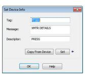
From the Device Info tab for the 1756-IF8IH and 1756-OF8IH Modules, Device Tag, Message and Descriptor can be configured.
