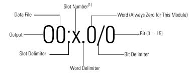
(1) I/O located on the controller (embedded I/O) is slot 0. I/O added to the controller (expansion I/O) begins with slot 1.
