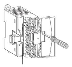
1. Route the wire under the terminal pressure plate.
