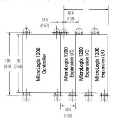
NOTE: All dimensions are in mm (inches). Hole spacing tolerance: ±0.4 mm (0.016 in.).
