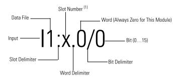
(1) I/O located on the controller (embedded I/O) is slot 0. I/O added to the controller (expansion I/O) begins with slot 1.
