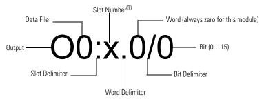
(1) I/O located on the controller (embedded I/O) is slot 0. I/O added to the controller (expansion I/O) begins with slot 1.
