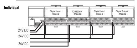
Wiring when total current draw is less than 10 A
