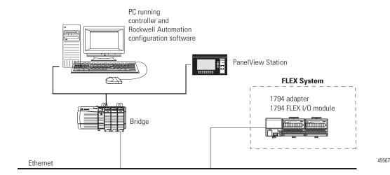
In this example, the FLEX I/O module communicates with the controller through the adapter. The controller can produce and consume tags. It can initiate MSG instructions that send and receive data or configure devices. Configuration of devices and the network is done through the personal computer running the controller and configuration software.
