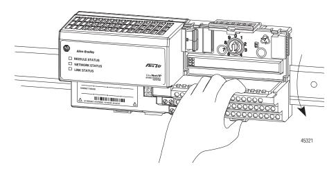
Gently push the FlexBus connector into the side of the adapter, or proceeding terminal base, to complete the backplane connection.
