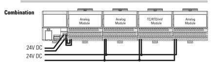
Total current draw through any base unit must not be greater than 10 A
