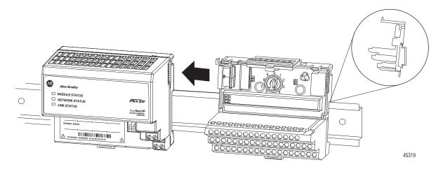
Make certain that the female FlexBus connector is fully retracted into the base unit.
