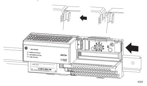
4. Slide the terminal base over tight against the adapter, or proceeding terminal base. Make sure the hook on the terminal base slides under the edge of the adapter, or proceeding terminal base, and the FlexBus connector is fully retracted.
