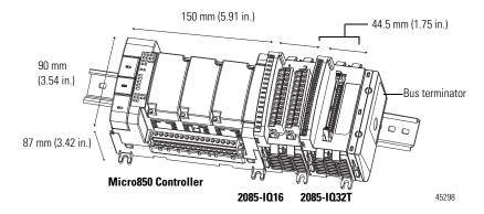
Mounting dimensions do not include mounting feet or DIN rail latches.
