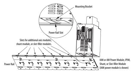
4. Pivot module downward and align the guide pins on the power rail with the guide pin holes in the back of the module.
