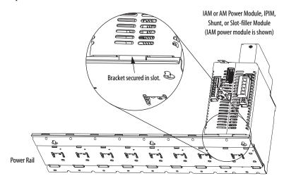
6. Use 2.26 N•m (20 lb•in) torque to tighten the mounting screws.
