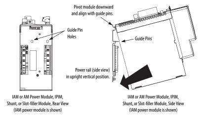
TIP The IAM module can have two or three power rail connectors and guide pins. The AM module can have one or two, all other modules have one.
