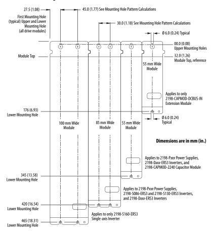
Also available to assist you with mounting holes is the Kinetix 5700 System Mounting Toolkit, catalog number 2198-K5700-MOUNTKIT.
