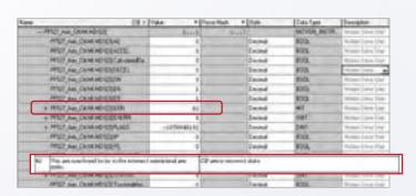
High quality diagnostic information is available through the generation of output instructions for each motor (axis). The instructions have built-in diagnostics including status of instruction execution and error codes.
