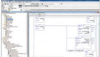
The PowerFlex 527 AC drive uses the same motion instruction set within Studio 5000 as Kinetix servo drives. The common user experience helps to simplify drive programming.
