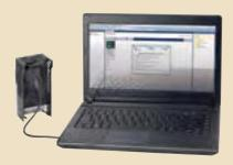
MainsFree™ programming allows configuration files to be uploaded and downloaded to the PowerFlex 525 and PowerFlex 523 drive control module via a USB connection.
