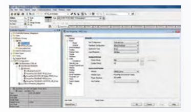
The PowerFlex 527 AC drive is configured as an axis of the machine using motions instructions within the Studio 5000 Logix Designer application. The configuration is stored in the Logix PAC.
