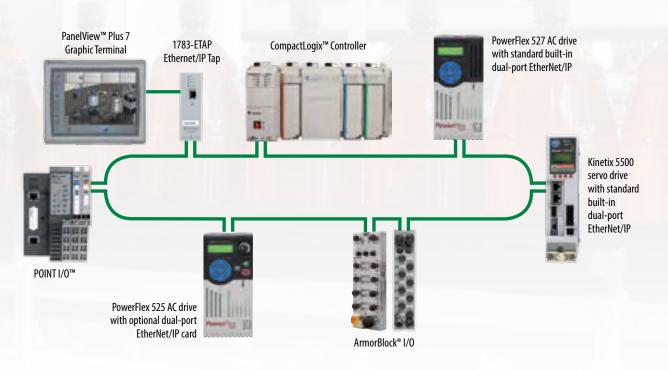
EtherNet/IP is an established, broadly adopted network that helps simplify and enhance machine design and operation. Dual-port EtherNet/IP connectivity supports linear and ring topologies as well as DLR functionality.
