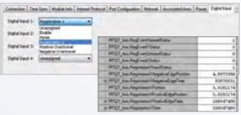
The ability to time stamp an input is crucial for data logging and regulatory compliance. With the use of motion instructions in the Studio 5000 Logix Designer application, fault and diagnostic information is easily made available in the software, with no additional configuration or messaging required.
