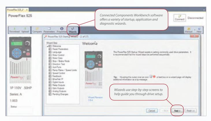
Connected Components Workbench software can help minimize your machine design and development time and is ideal for standalone applications. You can upload and download configurations over a USB connection and configure drives over EtherNet/IP, DeviceNet or other open industrial networks. Connected Components Workbench software supports PowerFlex drives as well as Micro800 programmable controllers and PanelView component graphic terminals.
