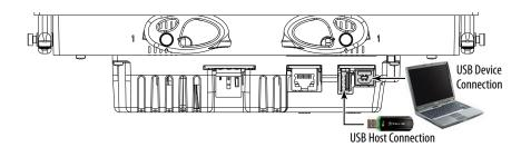
Icons identify the USB host connections. The USB host connection supports 0.5 A at 5V DC. Connected USB devices must not exceed this power load.
