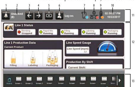
Here is an example of a screen in a project that is downloaded to the terminal.
