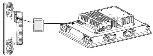
To remove the card, press the card so the retention feature releases the card, and pull out the card.
