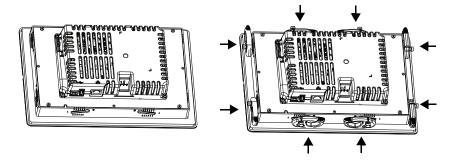
Each slot has six notches with alignment marks that are locking positions for a mounting lever. The thickness of the panel that you mount the terminal in determines the locking position that is required to maintain a NEMA, UL Type, and IP seal.
