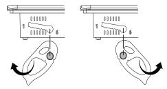
**4.** Slide and rotate each lever to a notch that is one or two positions greater than the final lock position. Start with the first lever in the sequence.
