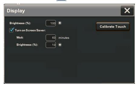
3. To add or remove the check mark next to Turn on Screen Saver, tap the checkbox.
