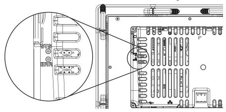
At startup, the STS and ERR indicators blink on and off, then the STS indicator blinks to signal progress during startup. If the indicators remain off, check the power cable.
