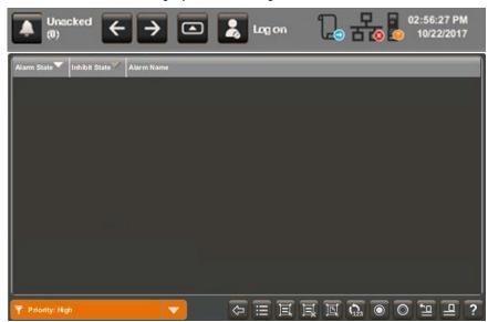
The selected filter displays in the filter pull-down menu.
