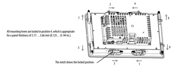
Figure 5 - Mounting Lever Orientation and Lock Sequence
