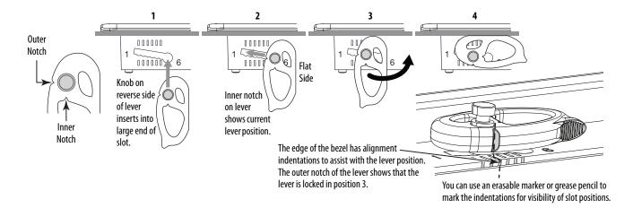
Initially, you secure the terminal in the panel by sliding each mounting lever to a position that is one or two notches greater than the final lock position. For example, if the final lock position is 1, slide each mounting lever to position 2 or 3. Follow the sequence specific to the terminal size shown in Figure 5 on page 28.
