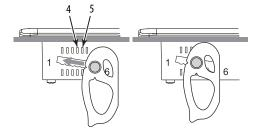
TIP To help position the levers and identify the final slot position, use the alignment marks or previous marks you made on the bezel.
