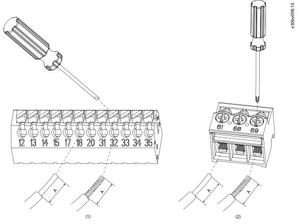
Figure 50: Inserting Wires into the Connector
