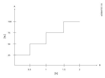
Figure 32: Reforming Procedure for DC Capacitors
