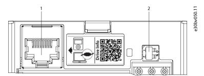
Figure 6: RJ45 Port and RS485 Termination Switch
