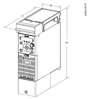
Figure 28: IP21/UL Type 1 Enclosure Sizes and Dimensions
