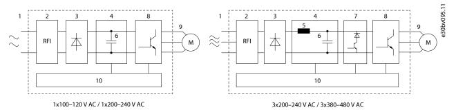
Figure 1: Block Diagram of iC2-Micro Frequency Converters
