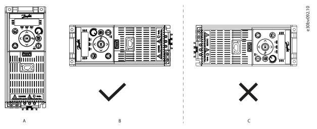
Figure 33: Mounting Directions for Drives
