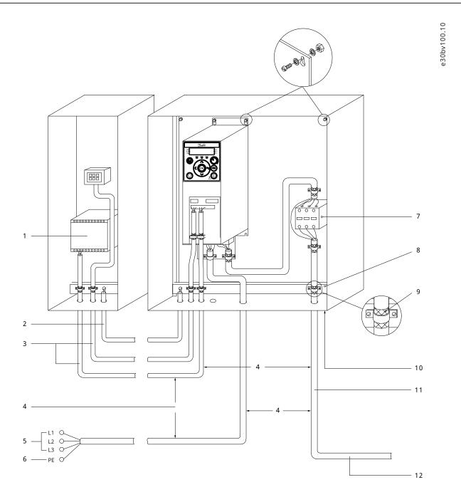
Figure 39: Example of Proper EMC Installation
