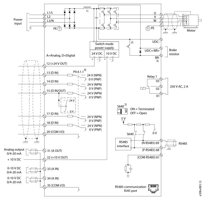
Figure 37: Wiring Diagram
