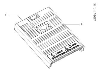
Figure 10: Sliding Door on the Terminal Cover
