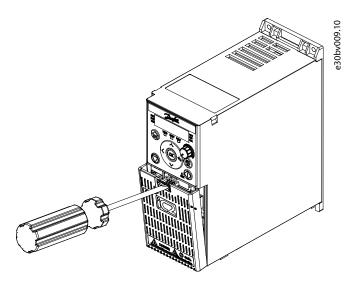
Figure 4: Removing Terminal Cover
