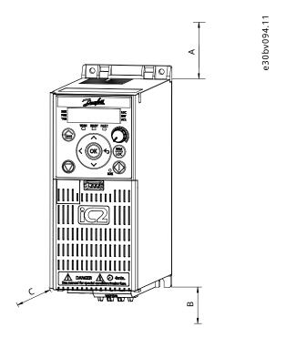
Figure 36: Recommended Clearance for Service Access
