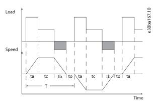
Figure 13: Typical Braking Cycle
