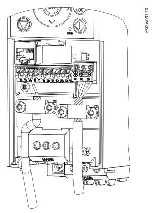
Figure 51: Correct Connection of the Cable Shield
