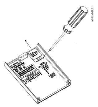
Figure 11: Removing the Sliding Door
