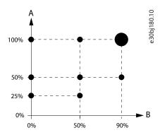
Figure 2: Operating Point According to IEC 61800-9-2 (EN 50598)
