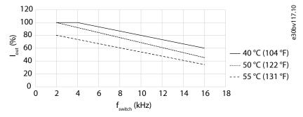
Figure 14: Derating of Output Current Versus Switching Frequency (MA01c 1x100–120 V AC and 1x200–240 V AC)
