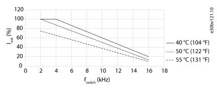
Figure 23: Derating of Output Current Versus Switching Frequency (MA02a 3x380-480 V AC)
