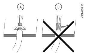
Figure 40: Installation of Cable Shield
