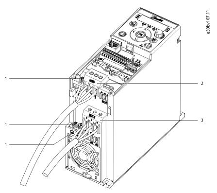
Figure 47: Mains, Motor, and Grounding Connection for 3-phase Units (Taking MA02a as an Example)
