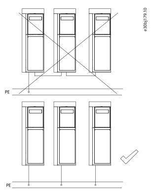
Figure 41: Grounding Principle
