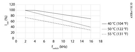
Figure 15: Derating of Output Current Versus Switching Frequency (MA02c 1x100-120 V AC and 1x200-240 V AC)
