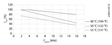
Figure 16: Derating of Output Current Versus Switching Frequency (MA02a 1x200-240 V AC)
