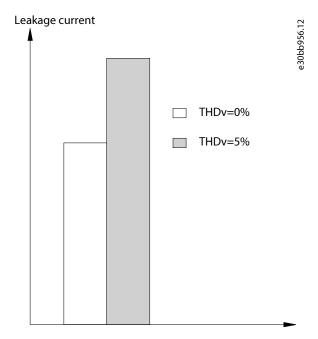
Figure 44: Influence of Line Distortion on Leakage Current
