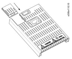
Figure 12: Installing the Sliding Door
