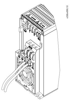
Figure 57: Connecting to Load Sharing and Brake
