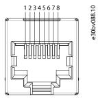
Figure 7: Pin Definition of RJ45
