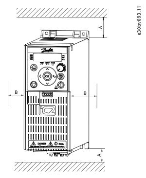
Figure 35: Minimum Clearance for Cooling
