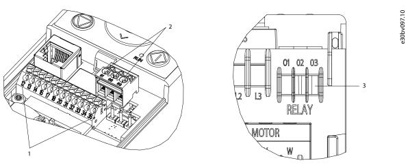
Figure 49: Control Terminal Numbers and Locations
