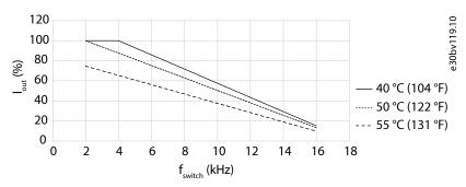
Figure 22: Derating of Output Current Versus Switching Frequency (MA01a 3x380–480 V AC)
