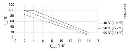
Figure 24: Derating of Output Current Versus Switching Frequency (MA03a 3x380-480 V AC)
