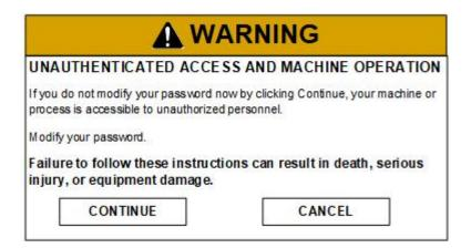
The default password must not be used. A new password must be defined after a password reset or at the first connection to the drive.
