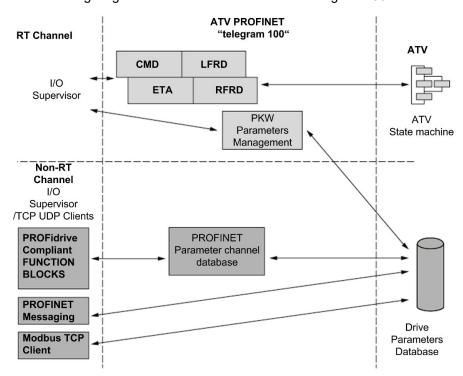
The PKW area of telegram 100, which is used for a simple parameter management, is compliant with the PKW mechanism used with the module.
