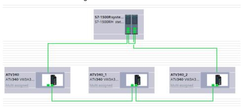
H-system with S2 redundancy: the synchronization between the two controllers is done via the fiber optical.
