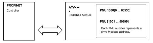
When the drive is operated in drive profile, the parameter management takes benefit of the PROFINET acyclic messaging features. With PROFINET, it is possible to exchange messages of variable length between both controllers (MS0 or MS1). These messages come in addition of the periodic data exchange.
