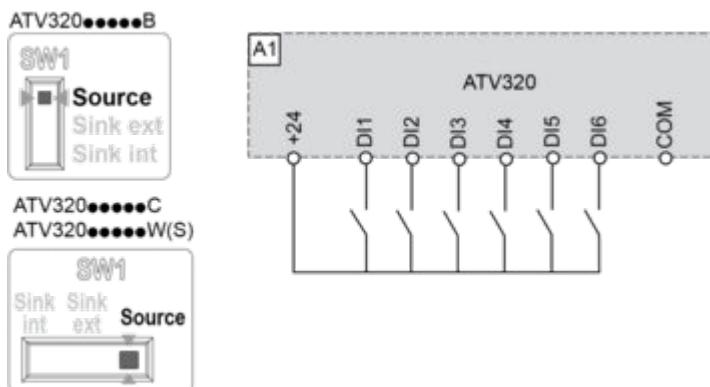
Switch SW1 set to "Source" position and use of an external power supply for the DI.
