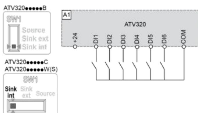
Switch SW1 set to "Sink Ext" position and use of an external power supply for the DI.
