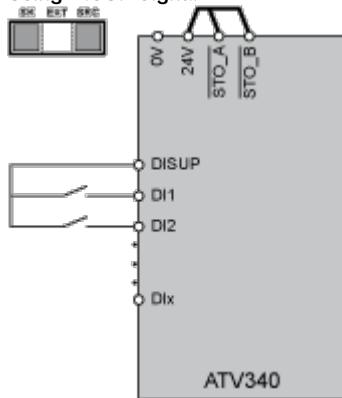
In SRC position DISUP outputs 24 V. In SK position DISUP is connected to 0 V.
