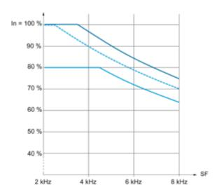
40 °C (104 °F) - Mounting type A, B and C 50 °C (122 °F) - Mounting type A and C 60 °C (140 °F) - Mounting type C
