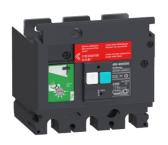
Earth-leakage add-on alarm module VigiPacT, ComPacT NSX 400/630, 200VAC to 440VAC, 30mA to 30A, 3 poles
