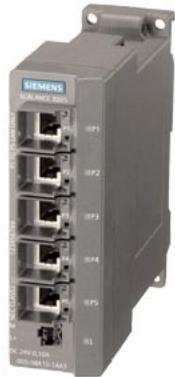
SCALANCE X005, IE Entry Level Switch unmanaged 5x 10/100 Mbit/s RJ45 ports, LED diagnostics, IP30, 24 V DC power supply, PROFINET-compliant securing collars, Extended temperature range -40 °C...+75 °C, Manual available as a download .
