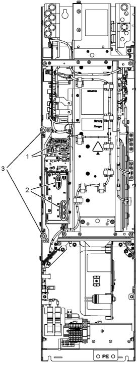
Figure 8-19 Replacing the Control Interface Board, Basic Line Module, frame size FB
