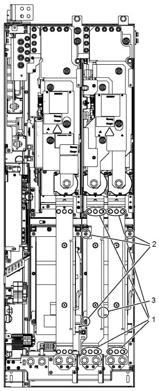
Figure 8-23 Replacing the fan, Smart Line Module, Active Line Module, and Motor Module, frame size HX - right power block
