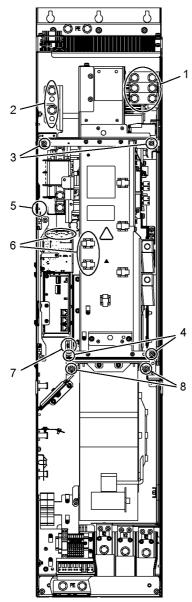
Figure 8-5 Replacing the power block, Smart Line Module, Active Line Module, and Motor Module, frame size GX
