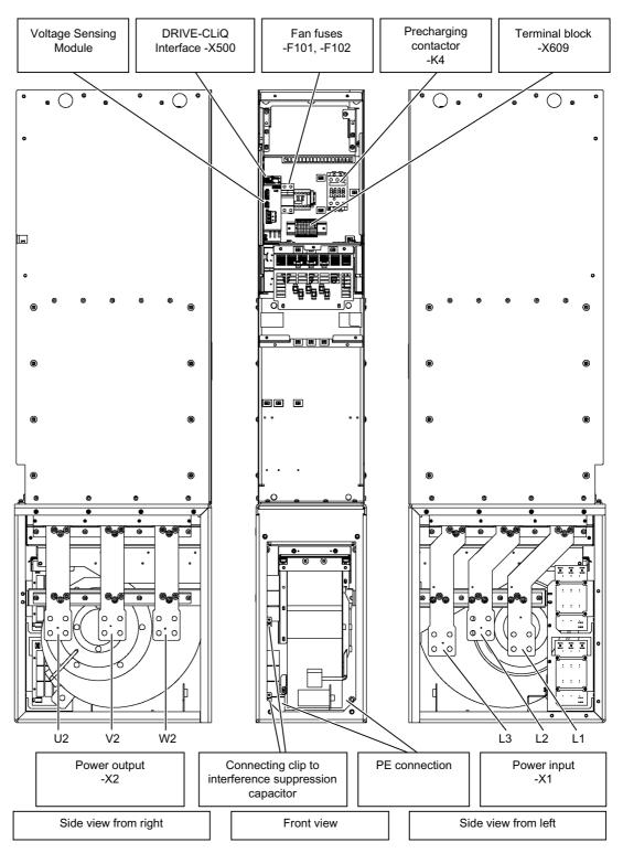
Figure 2-11 Interface overview in the Active Interface Module, frame size HI
