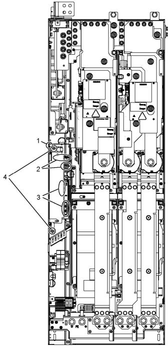
Figure 8-16 Replacing the Control Interface Board, Smart Line Module, Active Line Module, and Motor Module, frame size HX
