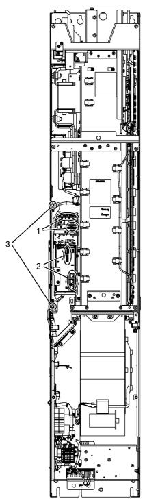
Figure 8-20 Replacing the Control Interface Board, Basic Line Module, frame size GB
