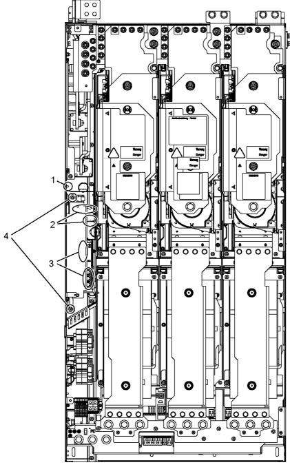
Figure 8-18 Replacing the Control Interface Board, Smart Line Module, Active Line Module, and Motor Module, frame size JX
