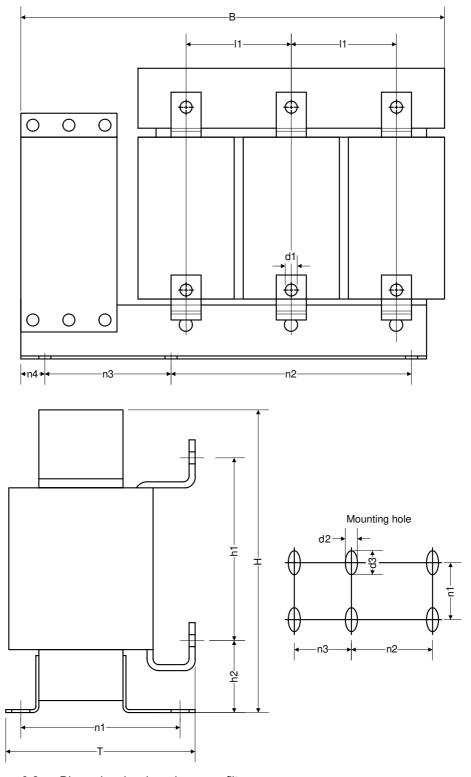
Figure 6-2 Dimension drawing, sine-wave filter
