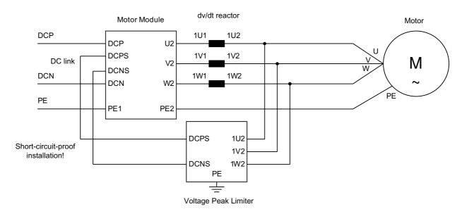
Figure 6-7 Connecting a dv/dt filter plus Voltage Peak Limiter for versions with one dv/dt reactor
