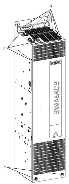
Figure 5-6 Installing the Braking Module in an Active Line Module / Motor Module, frame size FX – steps 1 - 3
