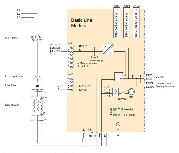
Figure 3-3 Connection example: Basic Line Module
