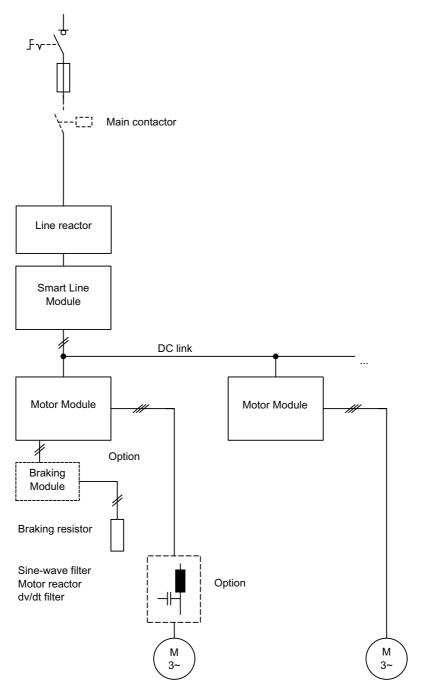
Figure 1-8 Basic structure of a drive system with SINAMICS S120 and unregulated infeed/regenerative feedback
