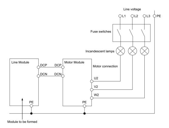
Figure 8-31 Forming circuit for Line Modules
