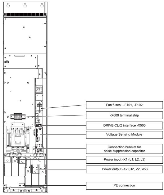
Figure 2-9 Interface overview in the Active Interface Module, frame size FI
