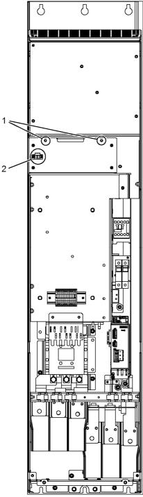
Figure 8-25 Replacing the fan, Active Interface Module, frame size FI
