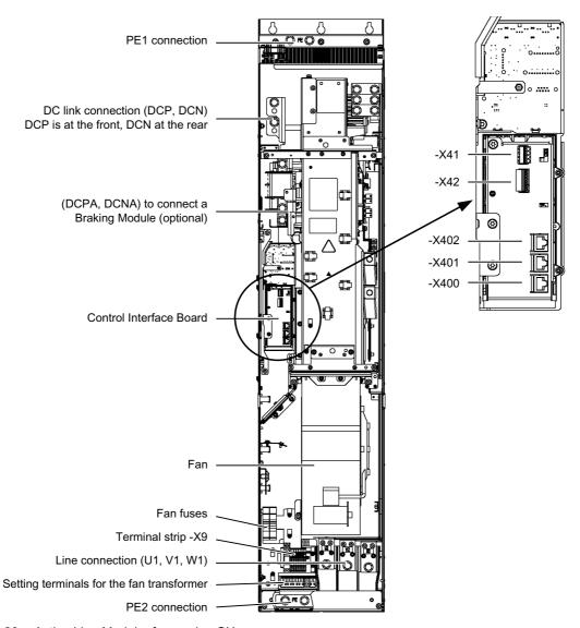
Figure 3-23 Active Line Module, frame size GX
