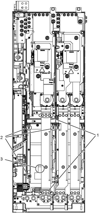
Figure 8-22 Replacing the fan, Smart Line Module, Active Line Module, and Motor Module, frame size HX - left power block
