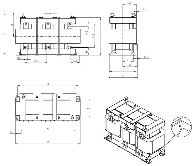
Figure 2-8 Dimension drawing of line reactor 6SL3000-0EH41-4AA0
