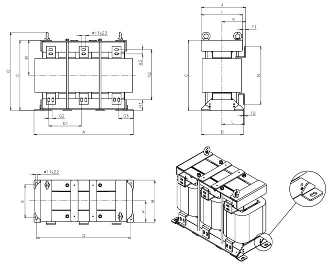
Figure 2-5 Dimension drawing of line reactor 6SL3000-0EE41-4AA0
