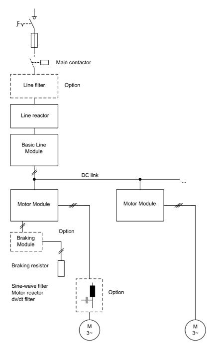
Figure 1-9 Basic structure of a drive system with SINAMICS S120 and unregulated infeed
