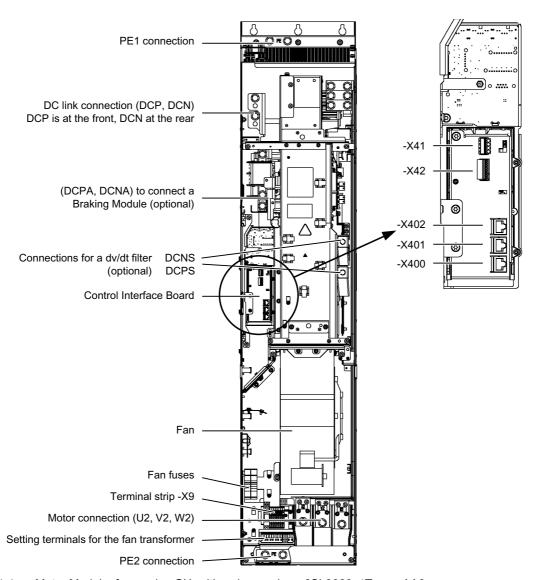
Figure 4-4 Motor Module, frame size GX, with order numbers 6SL3320–1Txxx–xAA0
