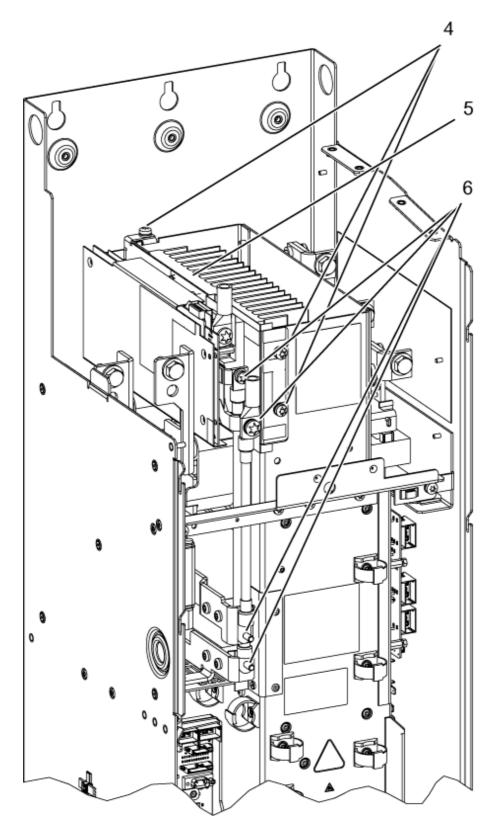
Figure 5-7 Installing the Braking Module in an Active Line Module / Motor Module, frame size FX – steps 4 - 6
