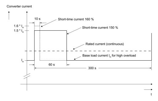
Figure 4-17 High overload
