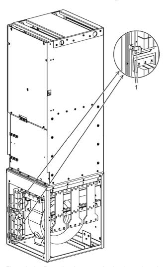
Figure 2-19 Removing the connection bracket to the noise suppression capacitor (example: frame size JI)
