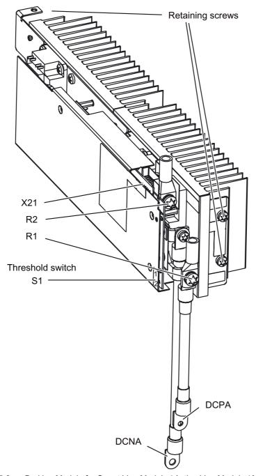
Figure 5-3 Braking Module for Smart Line Module / Active Line Module / Motor Module, frame size GX and for Basic Line Module, frame size GB
