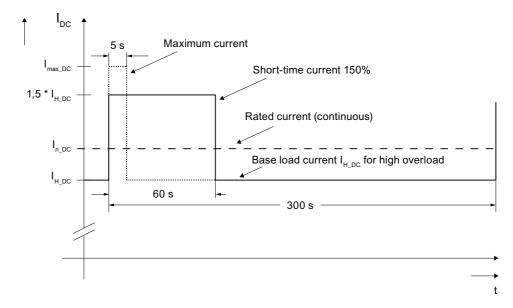
Figure 3-8 High overload
