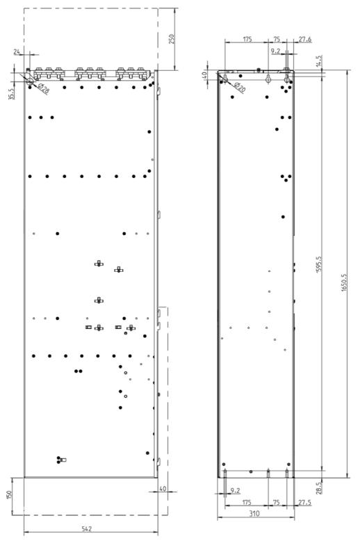
Figure 3-5 Dimension drawing, Basic Line Module, frame size GB Side view, rear view
