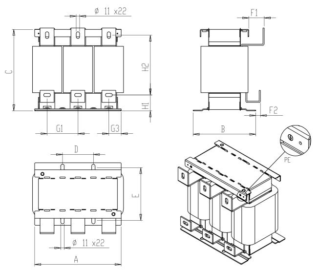
Figure 2-3 Dimension drawing of line reactor 6SL3000-0EE36-2AA0
