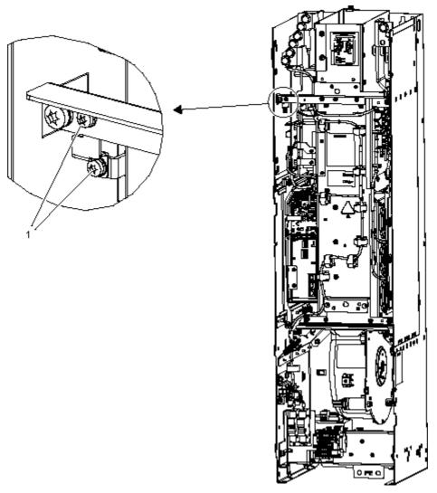
Figure 3-6 Removing the connection bracket to the noise suppression capacitor (example: frame size FB)
