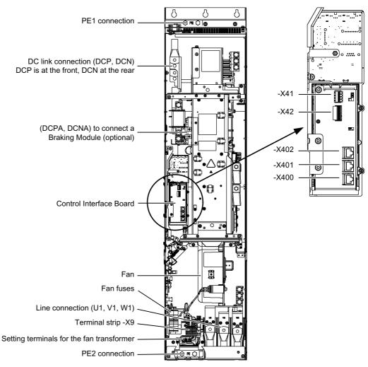
Figure 3-22 Active Line Module, frame size FX
