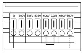
Figure 3-7 Setting terminals for the fan transformers (380 V – 480 V 3 AC / 500 V – 690 V 3 AC)
