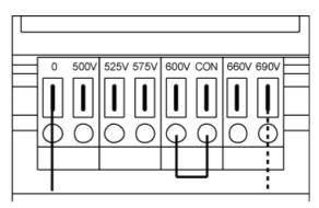
Figure 4-15 Setting terminals for the fan transformers (380 V - 480 V 3 AC / 500 V - 690 V 3 AC)
