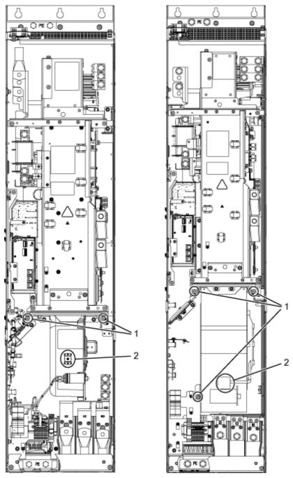
Figure 8-21 Replacing the fan, Smart Line Module, Active Line Module, and Motor Module, frame sizes FX, GX
