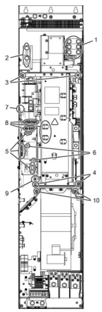
Figure 8-4 Replacing the power block, Motor Module, frame size GX
