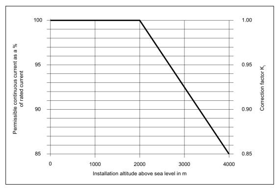
Figure 1-5 Current correction factor K<sub>T</sub> as a function of the installation altitude
