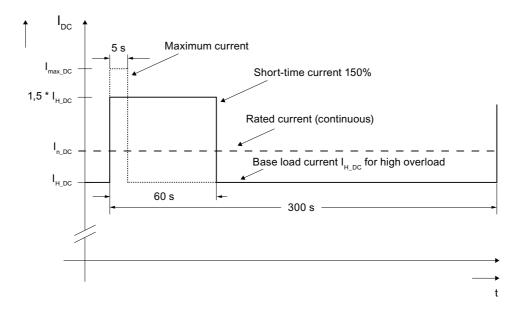
Figure 3-19 High overload
