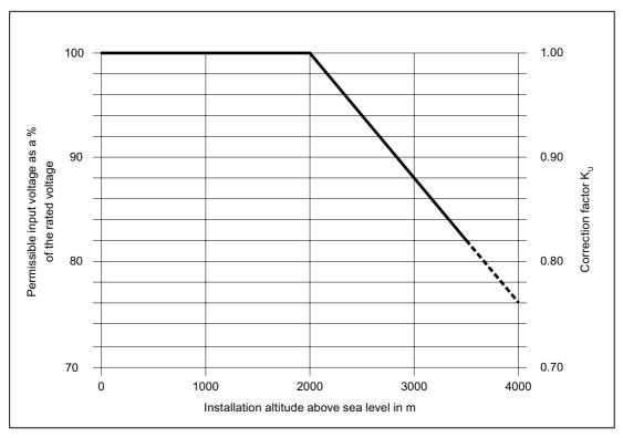
Figure 1-6 Voltage correction factor K<sub>T</sub> as a function of the installation altitude
