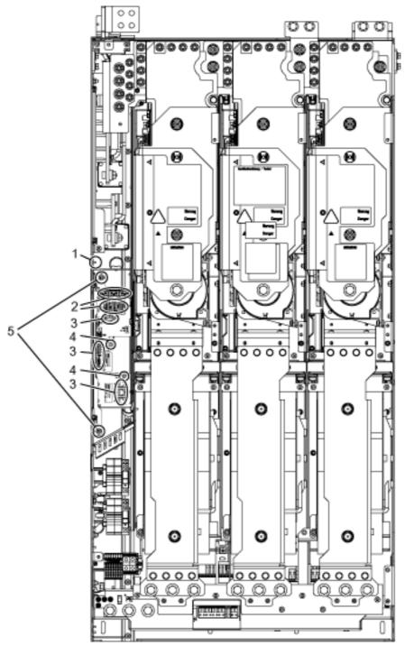
Figure 8-17 Replacing the Control Interface Module, Motor Module, frame size JX
