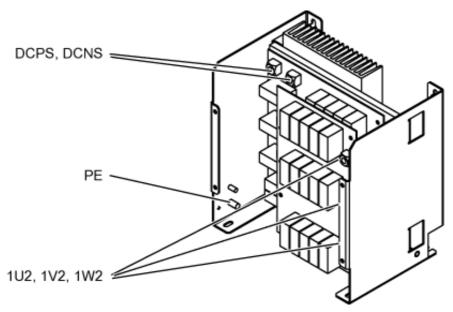
Figure 6-4 Interface overview, voltage peak limiter, type 1
