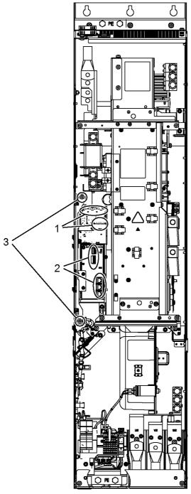
Figure 8-12 Replacing the Control Interface Board, Active Line Module and Motor Module, frame size FX
