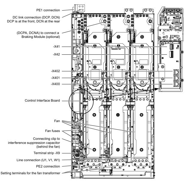
Figure 3-12 Smart Line Module, frame size JX
