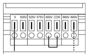
Figure 3-31 Setting terminals for the fan transformers (380 V – 480 V 3 AC / 500 V – 690 V 3 AC)
