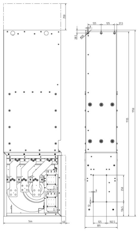
Figure 2-17 Dimension drawing for Active Interface Module, frame size HI Side view, rear view
