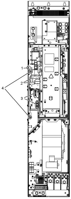
Figure 8-14 Replacing the Control Interface Board, Smart Line Module, Active Line Module, and Motor Module, frame size GX
