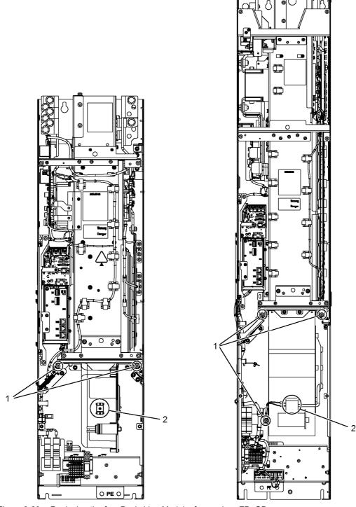
Figure 8-29 Replacing the fan, Basic Line Module, frame sizes FB, GB
