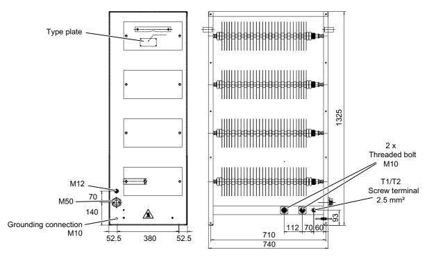
Figure 5-15 Dimension drawing braking resistor 50 kW/250 kW
