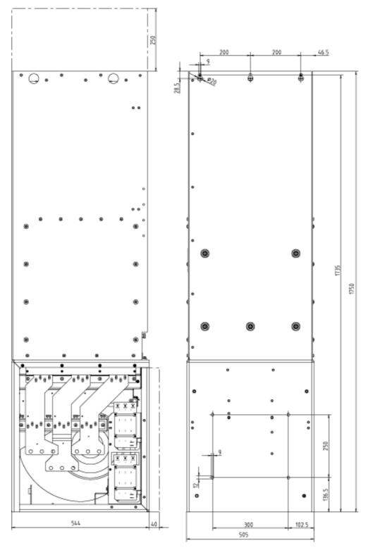
Figure 2-18 Dimension drawing for Active Interface Module, frame size JI Side view, rear view
