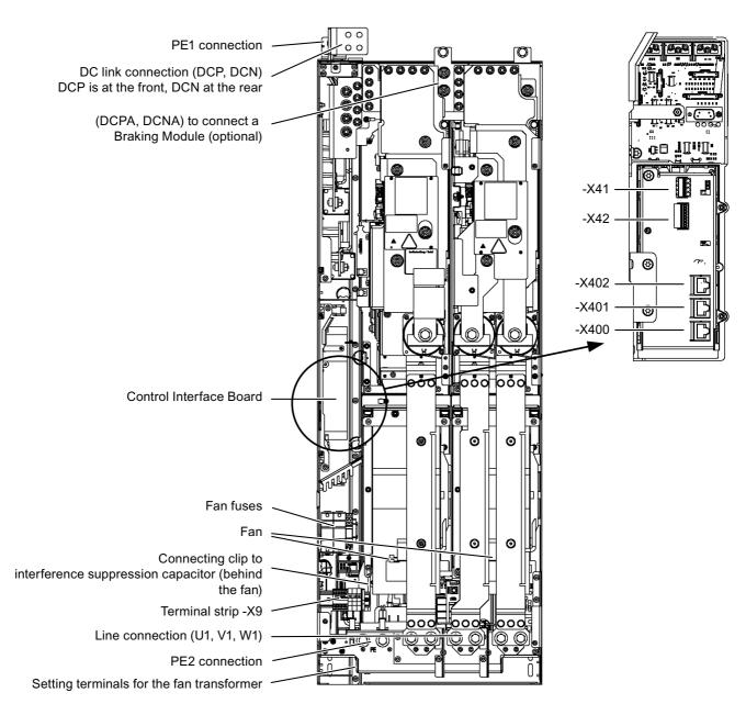
Figure 3-11 Smart Line Module, frame size HX
