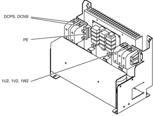
Figure 6-5 Interface overview, voltage peak limiter, type 2
