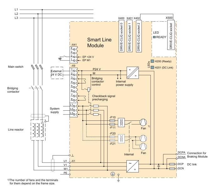
Figure 3-13 Smart Line Module wiring diagram
