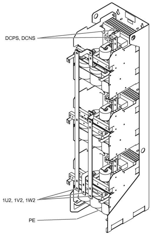
Figure 6-6 Interface overview, voltage peak limiter, type 3
