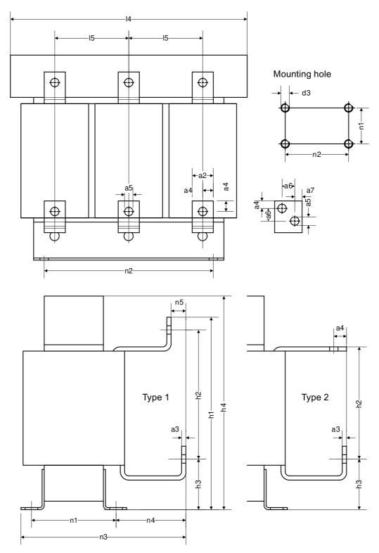
Figure 6-3 Dimension drawing, motor reactor
