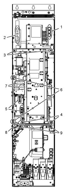
Figure 8-3 Replacing the power block, Active Line Module, and Motor Module (type FX)
