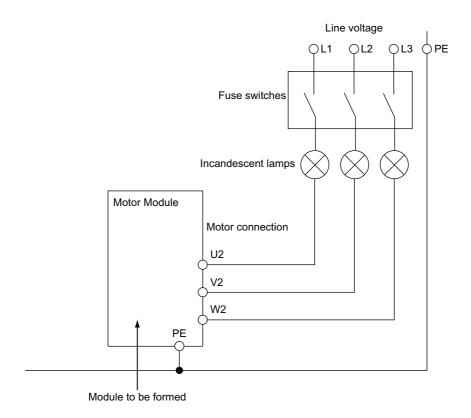
Figure 8-32 Forming circuit for Motor Modules
