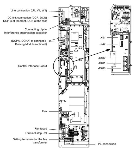
Figure 3-10 Smart Line Module, frame size GX
