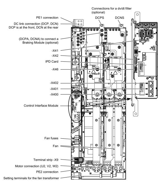
Figure 4-5 Motor Module, frame size HX, with order numbers 6SL3320–1Txxx–xAA3
