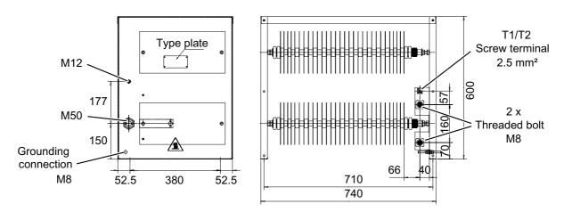
Figure 5-14 Dimension drawing braking resistor 25 kW/125 kW
