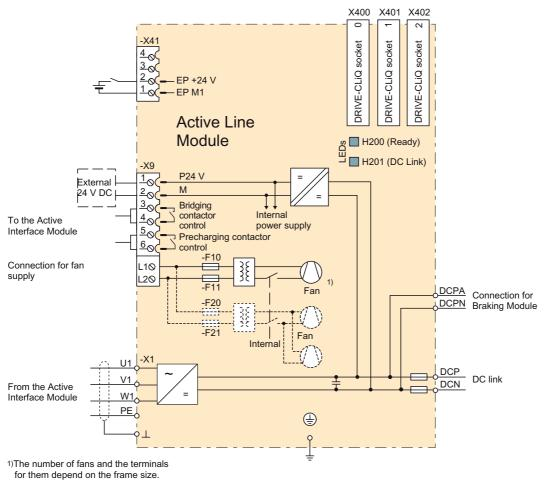
Figure 3-26 Active Line Module wiring diagram
