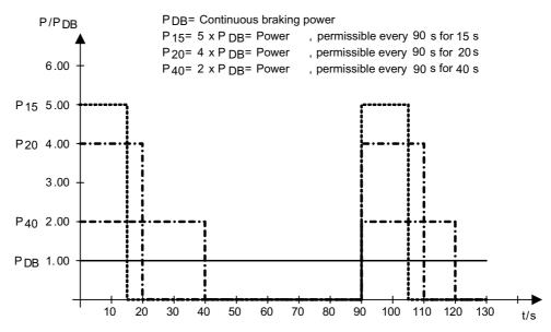
Figure 5-16 Duty cycle for braking resistors
