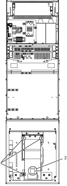
Figure 8-28 Replacing the fan, Active Interface Module, frame size JI
