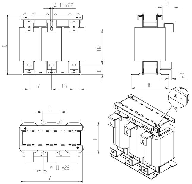
Figure 2-6 Dimension drawing of line reactor 6SL3000-0EH34-7AA0
