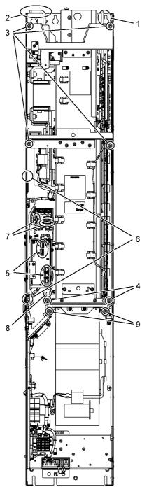
Figure 8-10 Replacing the power block, Basic Line Module, frame size GB
