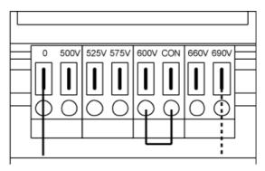
Figure 3-18 Setting terminals for the fan transformers (380 V – 480 V 3 AC / 500 V – 690 V 3 AC)
