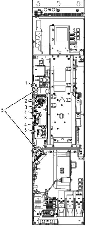
Figure 8-11 Replacing the Control Interface Module, Motor Module, frame size FX
