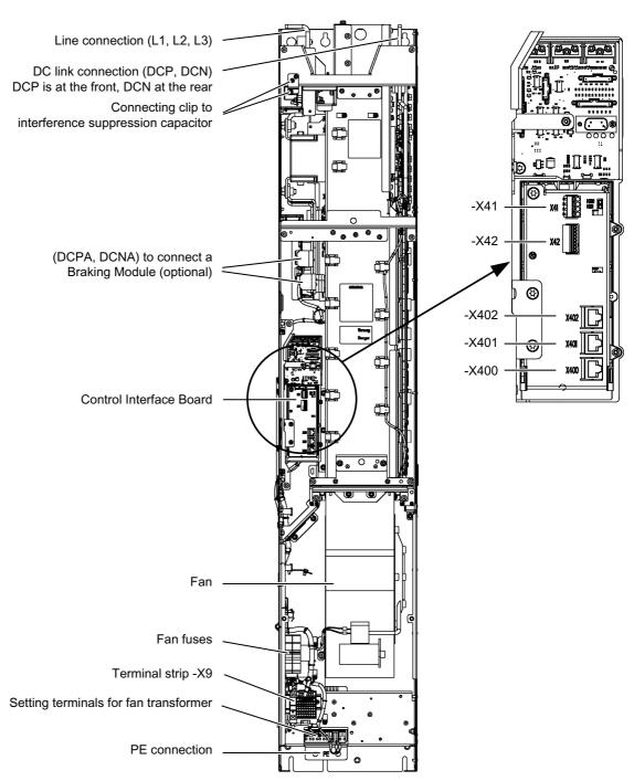
Figure 3-2 Basic Line Module, frame size GB
