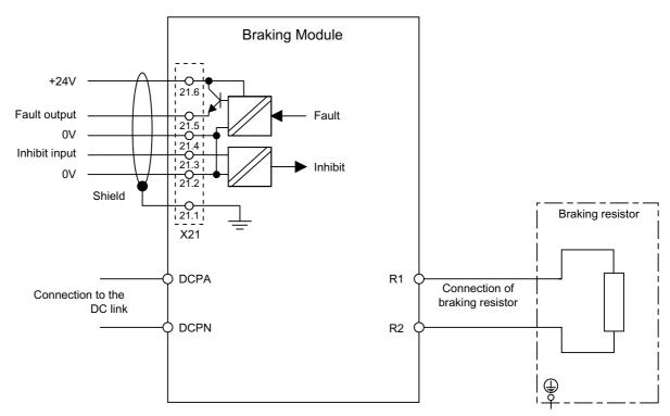
Figure 5-5 Connection example for Braking Module
