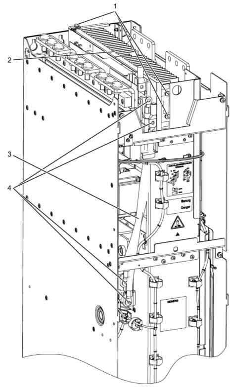
Figure 5-13 Installing the Braking Module in a Basic Line Module, frame size GB
