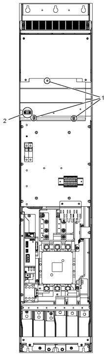
Figure 8-26 Replacing the fan, Active Interface Module, frame size GI
