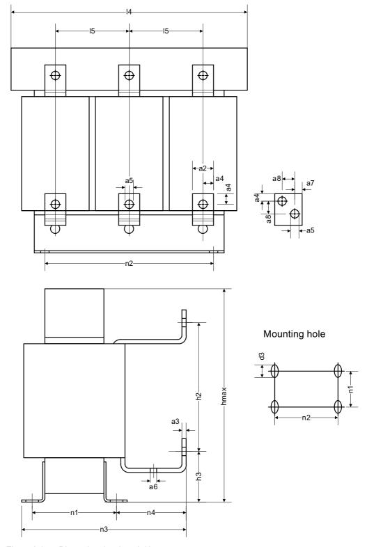
Figure 6-9 Dimension drawing, dv/dt reactor
