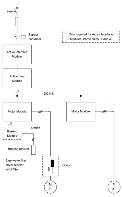
Figure 1-7 Basic structure of a drive system with SINAMICS S120 and regulated infeed
