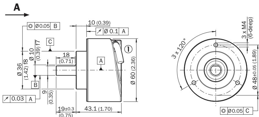
① Cable diameter = 5.6 mm +/- 0.2 mm bend radius = 30 mm
