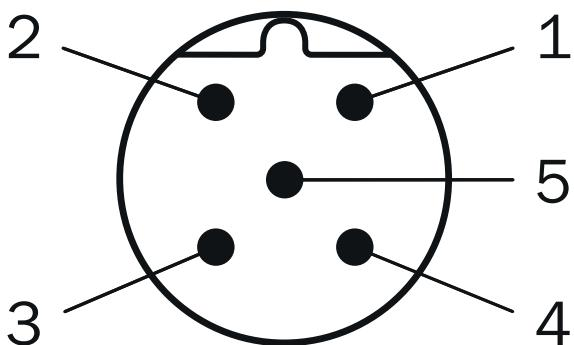
Male connector M12, 5-pin, A-coded
