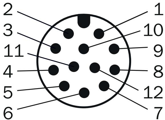
M12, 12-pin male connector, A-coded
