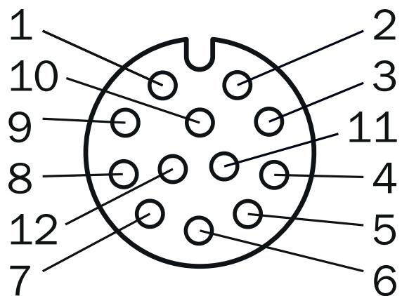
M12, 12-pin female connector, A-coded (I/O)
