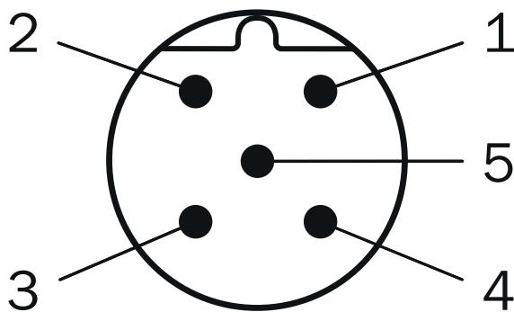
Male connector M12, 5-pin, A-coded
