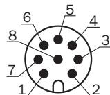
M12 male connector, 8-pin, A-coded
