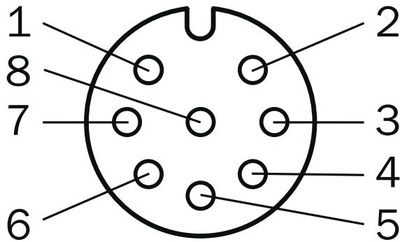
Female connector M12, 8-pin, A-coded
