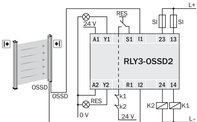
RLY3-OSSD2 at safety light curtain with automated reset and external device monitoring
