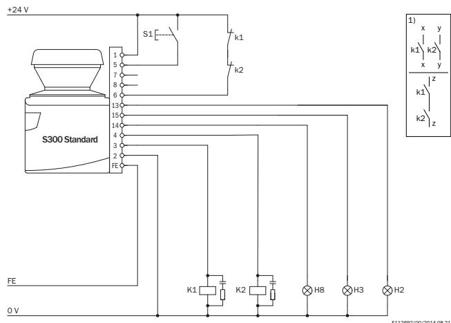
S300 Standard in conjunction with relays/contactors
