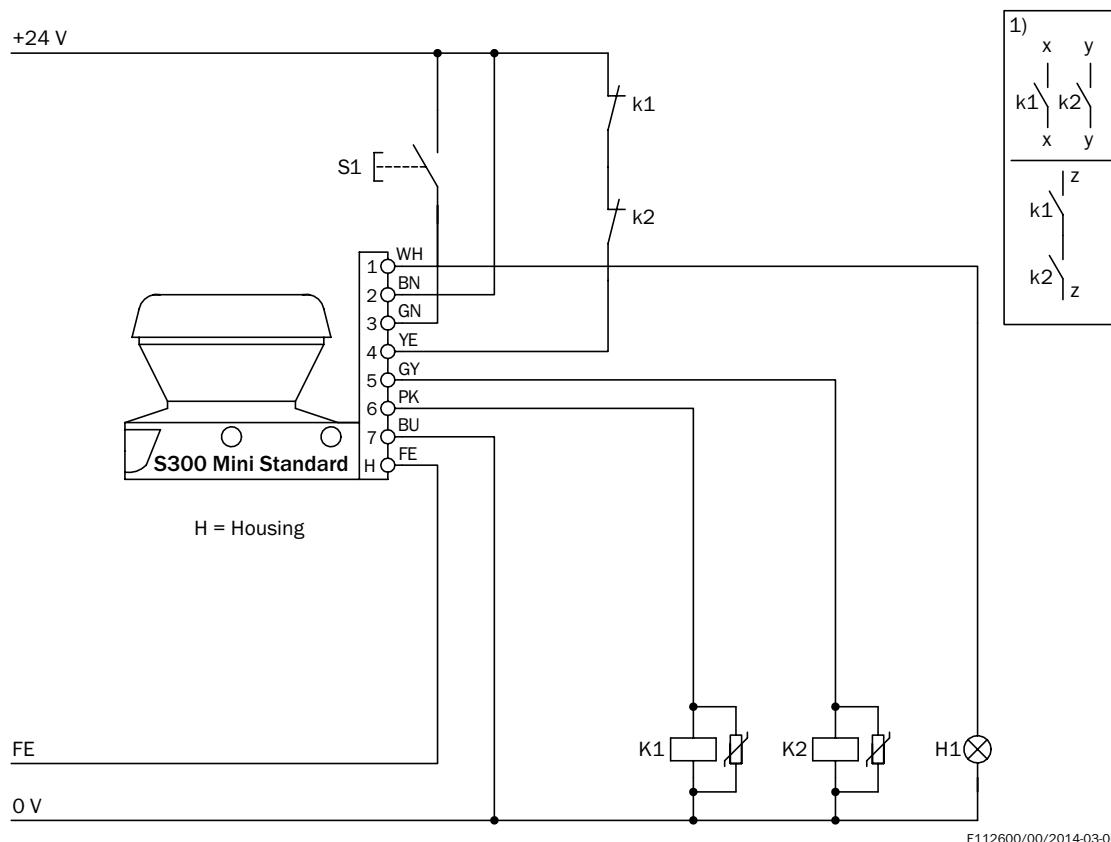
S300 Mini Standard in conjunction with relays/contactors
