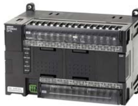
CP1L-EM CPU Units with 40 Points
