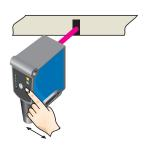
When setting the contrasts to be detected, the first LED (green) flashes in the bar graph. Press Teach-in pushbutton.
