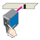
When setting the contrasts to be detected, the second LED (green) flashes in the bar graph. Press Teach-in pushbutton.
