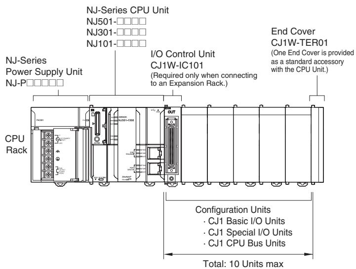
Even though the NJ-Series Controllers do not have Backplanes, the term "slot" still used to refer to the location of Units. Slot numbers are assigned in order to Units from left to right on the CPU Rack (slot 0, slot 1, slot 2, etc.).
