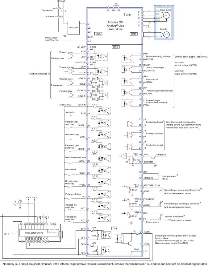
Normally B2 and B3 are short-circuited. If the internal regenerative resistor is insufficient, remove the wire between B2 and B3 and connect an external regenerative resistor between B1 and B2.
