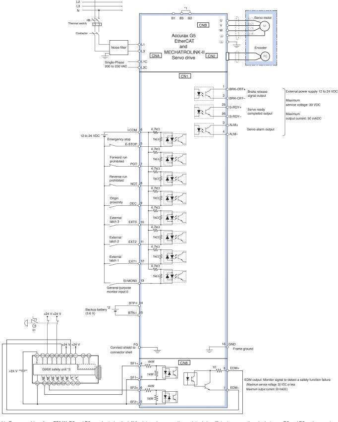
For servo drives from 750 W, B2 and B3 are short-circuited. If the internal regenerative resistor is insufficient, remove the wire between B2 and B3 and connect an external regenerative resistor between B1 and B2.
