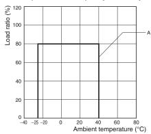
Note: 1. Set the parallel operation switch to the "PARALLEL" side (limit the rated output current to 80%).
