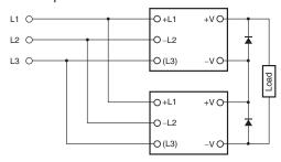
Note: 1. The diode is connected as shown in the figure. If the load is short-circuited, a reverse voltage will be generated inside the Power Supply. If this occurs the product may possibly deteriorate or be damaged. Always connect a diode as shown in the figure.
