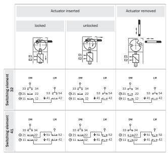
$<sup>\</sup>frac{1}{\mathbf{P}}$  Positive action N/C locking monitoring contact
