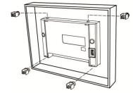
Step 3: Tighten the screws with the torque less than 0.5 N-M / 0.7 N-M to avoid damage to the plastic
