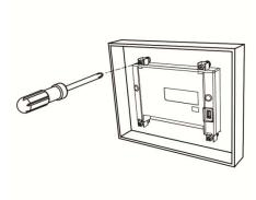
For heat dissipation, please keep a minimum clearance of 60 mm on the rear of the HMI.
