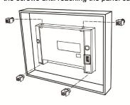
Step 4: For heat dissipation, please keep a minimum clearance of 60 mm on the rear of the HMI.
