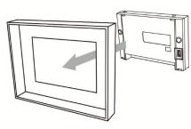
Step 3: Tighten the screws with the torque less than 0.5 N-M / 0.7 N-M to avoid damage to the plastic case.
