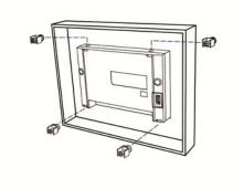
Place the fasteners into slots and tighten the
