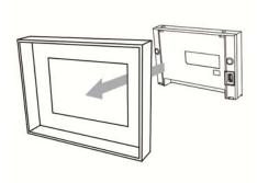
Step 3: Tighten the screws with torque less than 0.5N-M / For heat dissipation, please keep a minimum 0.7N-M to avoid damage to the plastic case. DOP-107/DOP-110 Torque: 6.17 lb-inch (0.7N-M) DOP-103 Torque: 4.41 lb-inch ( 0.5N-M )
