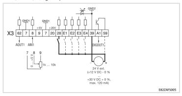
The min. wiring requirements for operation
