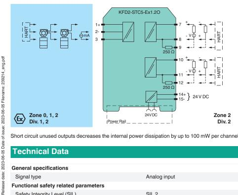
Short circuit unused outputs decreases the internal power dissipation by up to 100 mW per channel.
