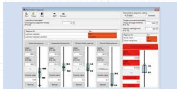
**Other features** It has convenient functions such as motor / driver information such as load factor, power supply voltage, driver temperature etc, logging function capable of recording interface recording, display function of non-rotating factors etc
