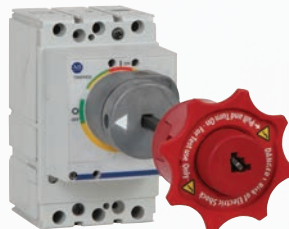
NFPA Internal Operating Handle – When using a variable depth operator allows for control of the MCCB with the enclosure door open without the use of tools.
