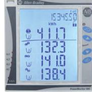
Equipped with an optional communication port, the unit communicates power and energy parameters to applications, such as FactoryTalk EnergyMetrix software. The power monitor works with these software applications to address these key customer applications:
