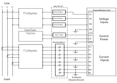
To find your specific wiring mode (Delta, WYE, Open Delta, Direct Connect) for PT configuration and CT configuration, refer to the following publications:
