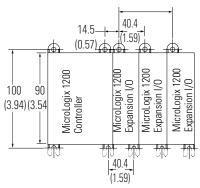
NOTE: All dimensions are in mm (inches). Hole spacing tolerance: ±0.4 mm (0.016 in.).
