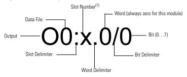
(1) I/O located on the controller (embedded I/O) is slot 0. I/O added to the controller (expansion I/O) begins with slot 1.
