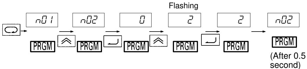
**Note 1.** If the new data is not to be registered, press the Mode Key instead of the Enter Key. The new data becomes invalid and the constant no. display (“n02”) is returned.
