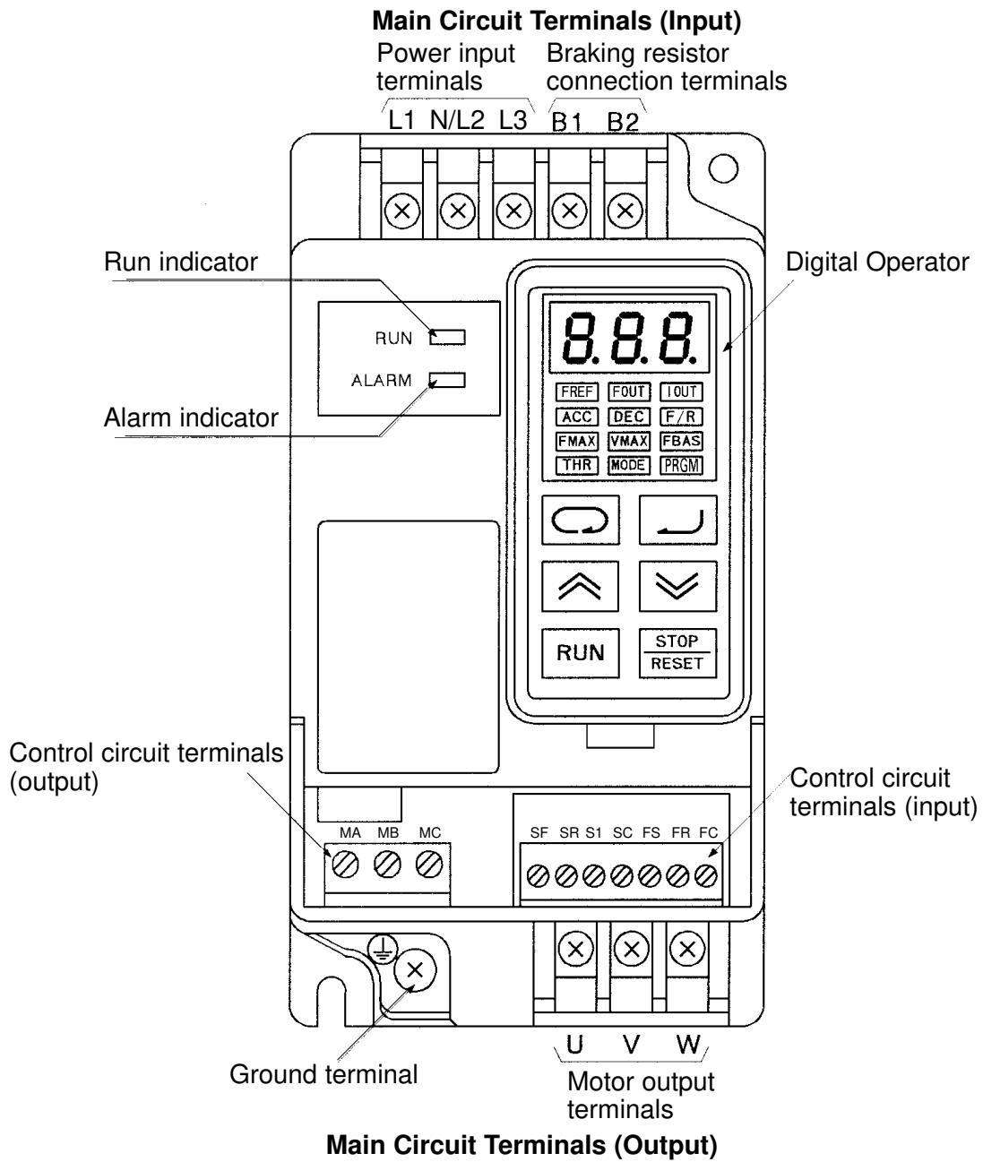
**Note** This diagram shows the Inverter with all terminal block covers removed.
