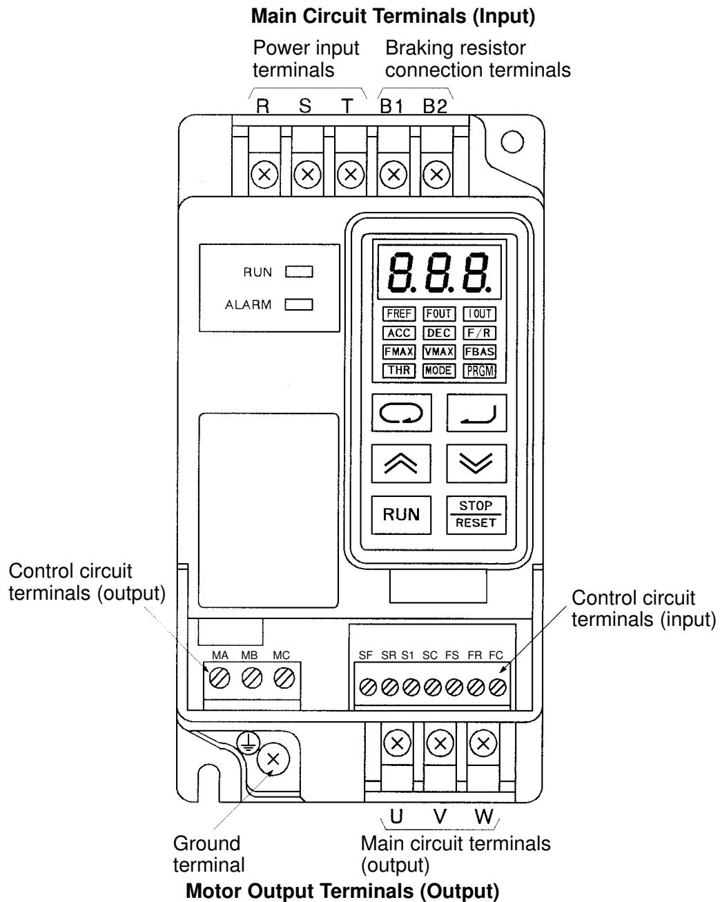
**Note** This diagram shows an Inverter with all terminal block covers removed.
