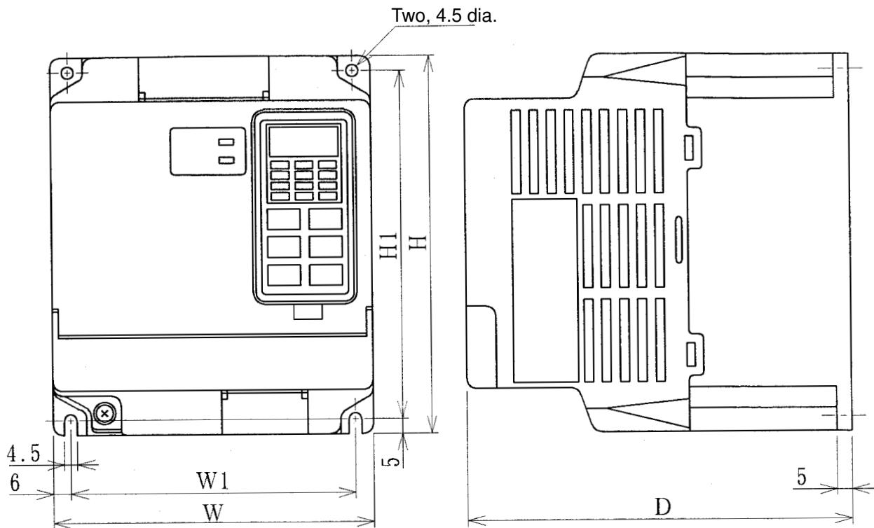
**Note** Install the Inverter with four M4 bolts.
