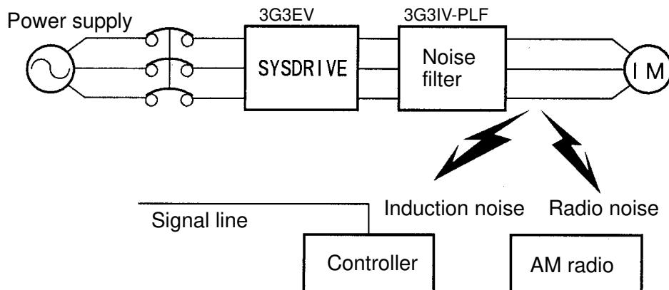
**Induction Noise:** Electromagnetic induction generates noise on the signal line, causing the controller to malfunction.
