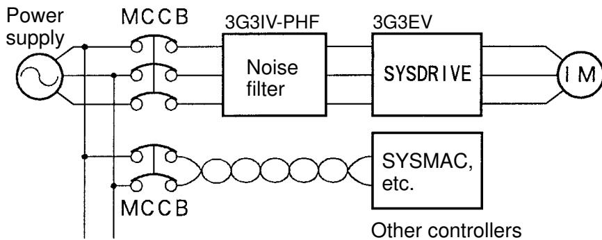
**Note** Use a special-purpose noise filter for Inverters.
