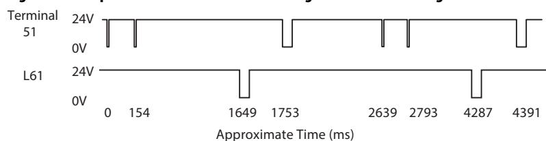
Figure 28 - Output Pulse Test Pattern for Two High Side Guard Locking
