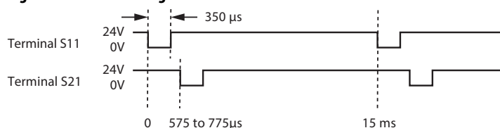
Figure 24 - Pulse Test Signals
