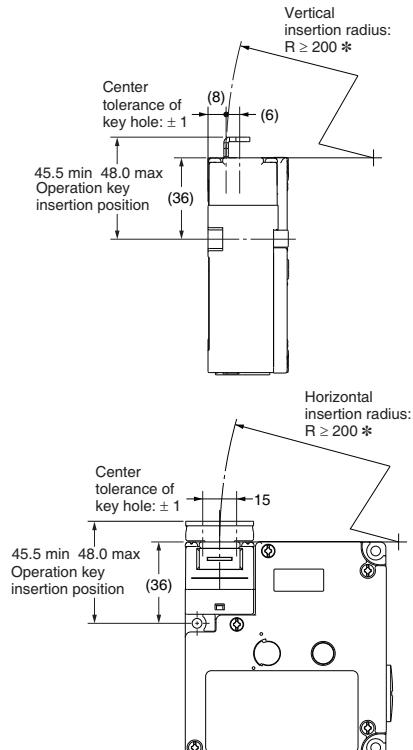
\* Insertion radii apply when the rotational center of the Operation Key is in line with a line extending from the front or top Head surface.
