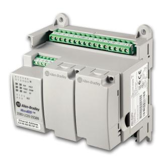
The new Allen-Bradley Micro820 20pt controller is specifically designed for small standalone machines and remote automation projects with embedded Ethernet and Serial ports. It can function as a RTU (remote terminal unit) for remote machines with support for Modbus RTU and TCP. It has embedded support for 4 thermistor temperature inputs for use as a DDC (direct digital controller) for Building Management Systems.
