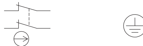
Figure 96 - Contact Opening Characteristics
