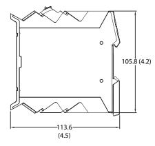
Position the interface module on an IEC standard (35 x 7.5 x 1 mm) top-hat DIN rail at a slight angle (DIN rail: Allen-Bradley part number 199-DR1; 46277-3; EN50022).
