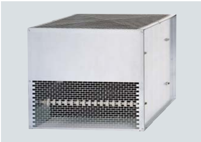
Example: Braking resistor for PM240 Power Modules frame size FSGX Excess energy in the DC link is dissipated in the braking resistor. The braking resistors are intended for use with PM240 Power Modules which feature an integrated brake chopper, but cannot regenerate energy to the supply system. There is an optional plug-in Braking Module for frame size FSGX. For generator operation, e.g. the braking of a rotating mass with high moment of inertia, a braking resistor must be connected to convert the resulting energy into heat.
